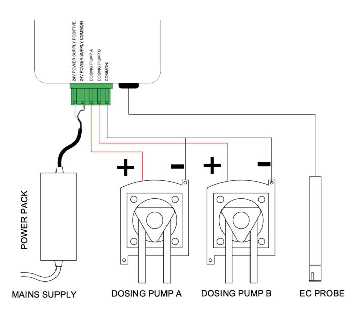
Note: that all the connections marked 24V Common are connected internally and you may connect the return wire from any solenoid valve or pump to any of these commons. The 24V live wire is normally marked by a white stripe or white printing along its length.
