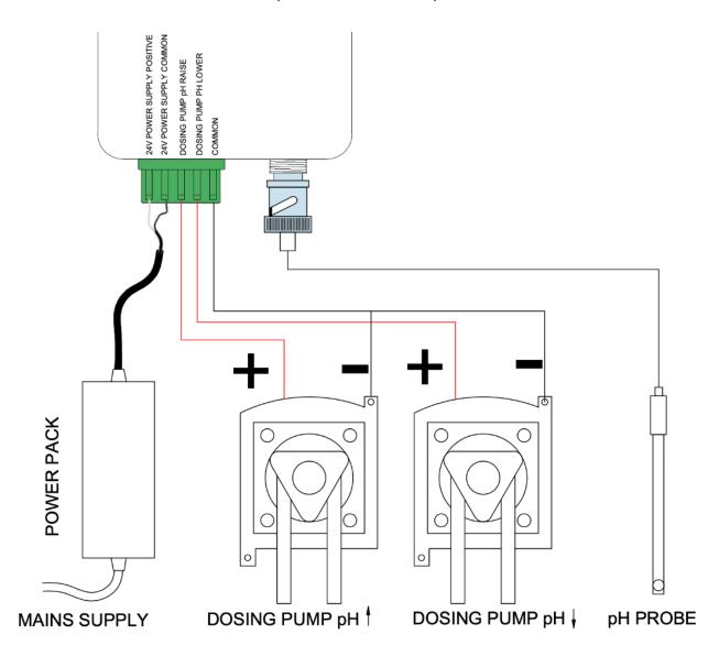
Note: that all the connections marked 24V Common are connected internally and you may connect the return wire from any pump to any of these commons. The 24V live wire is normally marked by a white stripe or white printing along its length.
