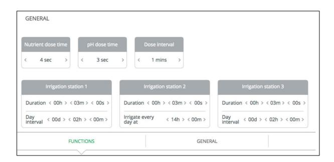
When using single output or sequential irrigation then only one irrigation trigger can be specified.
