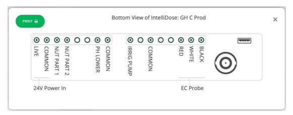
The low voltage power from the adapter is connected to the two-left connection terminals on the left-hand connector. With many power supplies, the cable is a screened "co-axial" type. In this case the screen should be connected to the "Common" and the centre wire to the 24V line connection on the controller.
