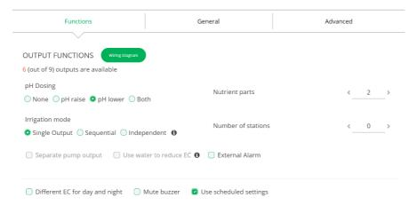
To set up the scheduling function, scroll down the page to Functions and tick the "Use scheduled settings".
